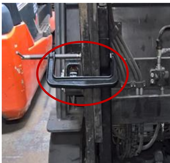
G-Clamp securing prop
