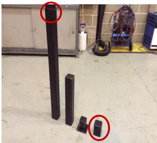
End cap must be fitted
